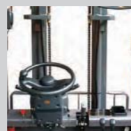
The wide mast, low scuttle and high seating position gives the operator an excellent view, reduces loading damage and accidents.
