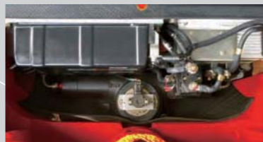
The state-of-the-art controller can be easily accessed at waist height, helping to reduce servicing time. AC technology to heavy-duty applications. The use of current is optimised and AC motors are brushless, which minimises servicing. Motors are very well protected against the water and dust. Roll-back is almost eliminated and higher travel speeds are attainable. More than thirty performance parameters can be adjusted to suit all type of load, working area and skill of the driver.
