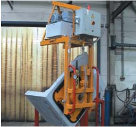
Vacuum Lifting Device with 180° Turning Unit
