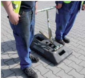
Site Fence Base Handle BZSH
