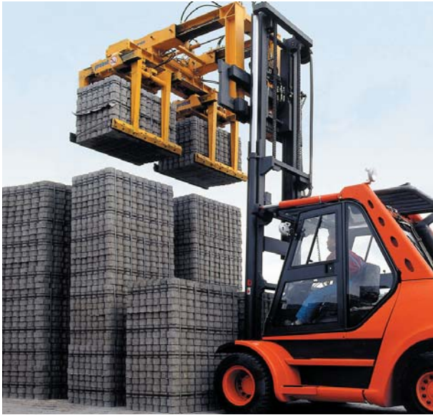
Double Grab with Telescopic Crane Boom STAZ-DZ-II
