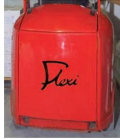
Detailed steel plate rear panel protects traction battery. Narrow 1000mm wide rear chassis allows block stacking and drive in rack operation.
