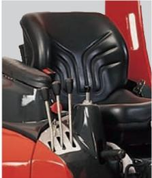
High quality adjustable full suspension seat with operators lumbar support.
