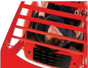
The unique 'Hi Vis' twin cost safety guard combines maximum visibility and overhead protection for the operator.
