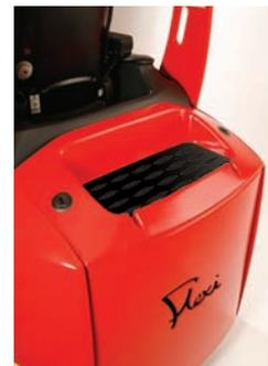
Conveniently located behind the operator and suitable for carrying a roll of plastic film or any other material that needs to be close to hand.
