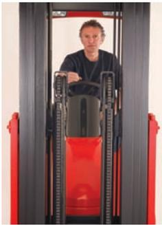
Operators have excellent forward visibility thanks to the triplex free lift mast, with its twin side mounted lift cylinders. Mast tilt means easy fork entry into pallets – even over trailer retaining rails.
