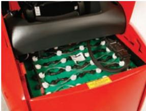
Low rear lift off or roll off for fast changeovers. Good access for battery topping. No motors underneath.
