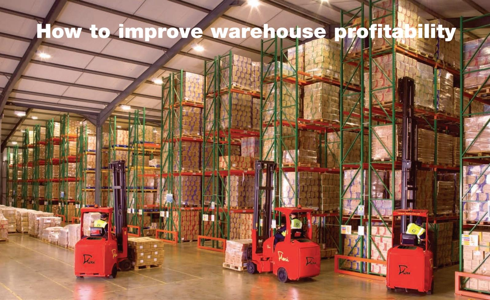
**Flexi** works in just 1600mm (ISO)\* or 1800mm (EURO)\* aisle widths - liberating a potential **30% more** warehouse capacity compared with conventional reach trucks.
