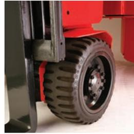
Four large cushion rubber tyres deliver optimum performance and traction in loading yard. They're also resistant to damage which means a long service life and less downtime.
