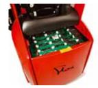
Low lift off or roll off for fast changes. Clear battery access with no components or motors underneath.
