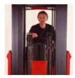
FLEXI operators have excellent viibility thanks to a 'Hi Vis' lift mast which has twin side mounted free lift cylinders.
