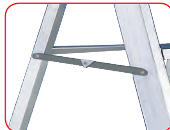
Anti-closing / opening bars in galvanized steel. In addition to avoiding accidental opening or closing, they reinforce the ladder in the central part. Ideal for industrial use where the anti-opening straps are damaged more easily.
