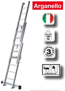
Extension ladder in three sections with a winch mechanism. Extruded aluminum ribbed profiles. It has a gear and pulleys to open and close the 2 upper sections to lean the ladder to the wall. Equipped with wall wheels at the end of the last section. Equipped with anti-slip feet.
