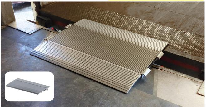
DPC aluiminum mobile bridge, unlike PLQ, is engineered with H40 ALUMINUM EXTRUDED PROFILES, this means it's SUITABLE WITH HEAVIER LOADS (up to 6T). The extrusion architecture causes the ramp to become a NATURAL BUMP, so this ramp is SUITABLE WITH BIG WHEELED VEHICLES (LIKE CABINED FORKLIFTS).
