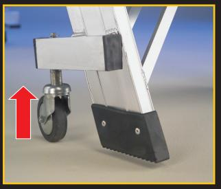
As soon as the user mounts the ladder, the springs compress allowing both the front and the back rubber feet to touch the ground, firmly blocking and braking the ladder with no need for other devices.
