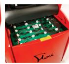
Complete new battery and tank installed. Low energy charger supplied.
