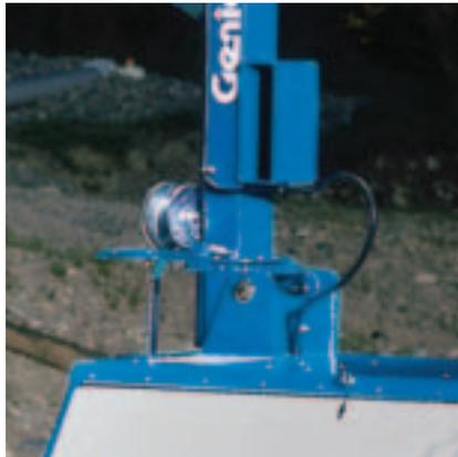
Easy to use winches are mounted high on the machine, allowing the operator to stand upright while raising/lowering the mast.
