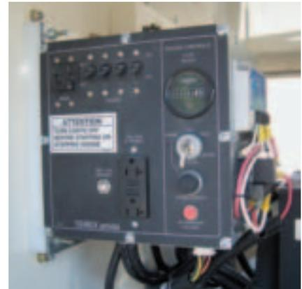
Control box shown with optional Roda Deaco electronic air shutdown system (model AL5000).
